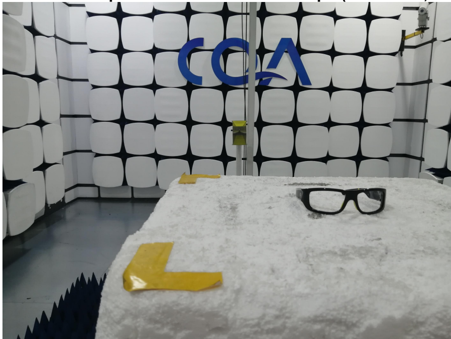
Radiated spurious emission Test Setup-2(Above 1GHz)
