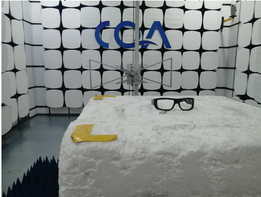
Radiated spurious emission Test Setup-1(Below 1GHz)
