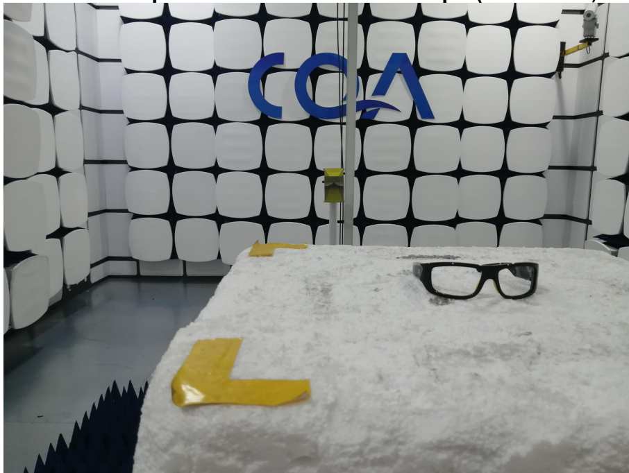
Radiated spurious emission Test Setup-2(Above 1GHz)
