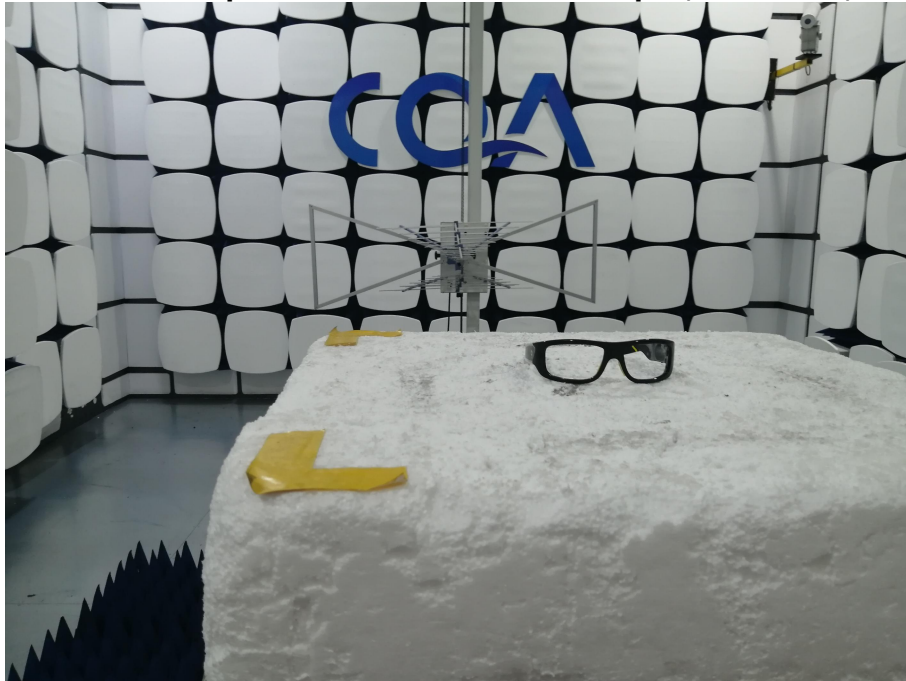
Radiated spurious emission Test Setup-1(Below 1GHz)
