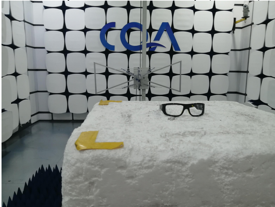
Radiated spurious emission Test Setup-1(Below 1GHz)
