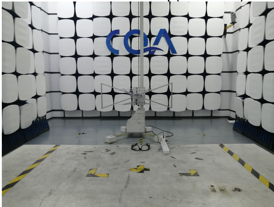
Radiated emission Test Setup (30MHz~1GHz)
